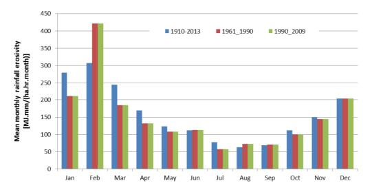
Figure 6: Monthly mean rainfall erosivity (MJ.mm.ha<sup>-1</sup>.hr<sup>-1</sup>.month<sup>-1</sup>) in three historical periods from BoM data
