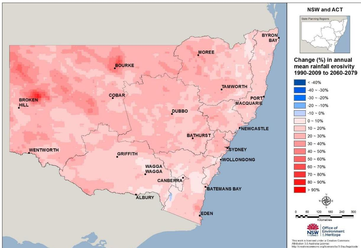
Figure 13: The percent change in rainfall erosivity in the far future (2060–2079) compared with the baseline period (1990–2009)
