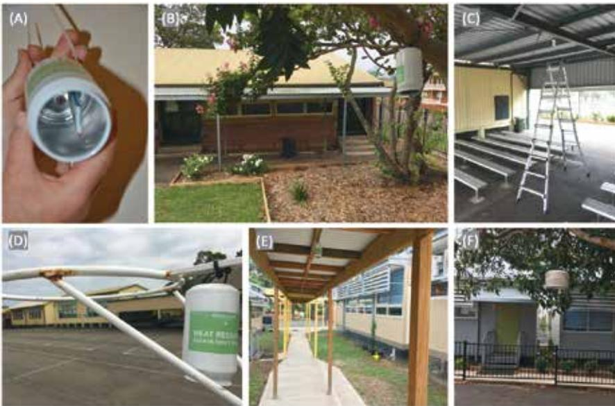
**FIGURE 8:** Image of the two devices used for collection of permanent air temperature information. (A) Mounting the Tempmate® sensor into the protective shield. (B-E) Heat logger at several locations across the school (red diamonds A, C, F and L in Fig. 5). (F) Stevenson screen containing a TinyTag logger (yellow square in Fig. 5). Image© S. Pfautsch.
