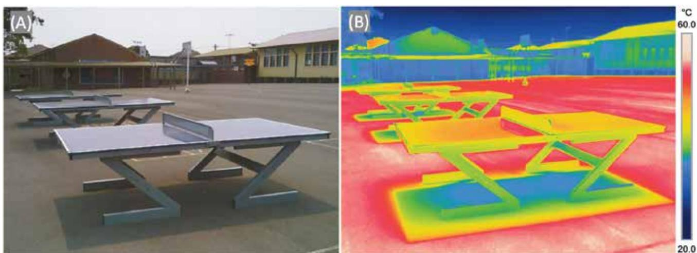
**FIGURE 10:** Example of a normal view and infrared view of the ping-pong tables in the central school yard. The image was taken during the afternoon in full sunshine (30 December 2019). Surface temperatures of the tables was 48.5°C, asphalt in the sun was up to 56°C, while in the shade underneath the tables around 37°C, highlighting the pronounced cooling effect of shade on dark surfaces (a difference of 19°C). Image© S. Pfautsch.
