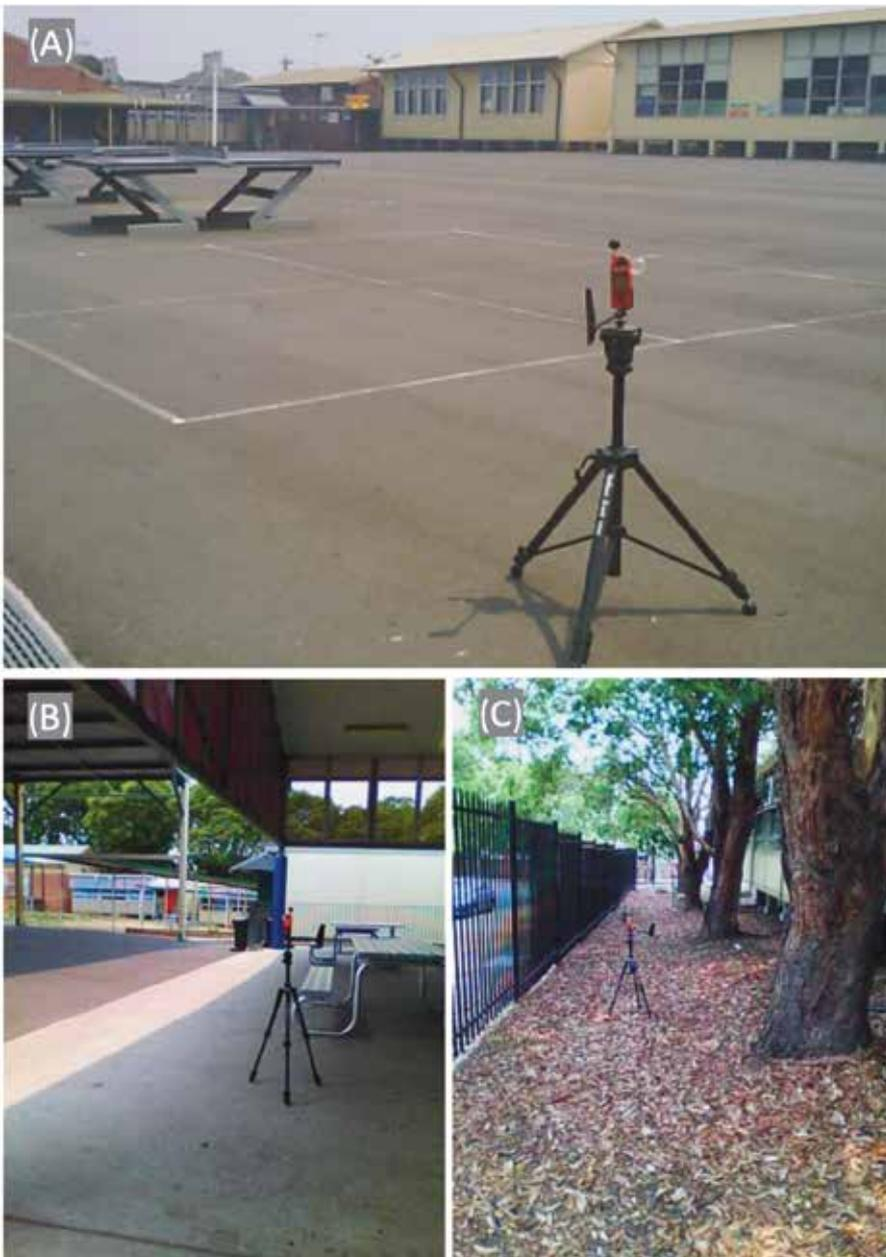
**FIGURE 9:** Recording of black globe temperatures (TBG) using the micrometeorological weather station. (A) Central school yard on asphalt in full sun. (B) At the entrance of the communal hall on concrete in the shade. (C) Tree grove at the western fence on dry grass and leaves in the shade. Image© L. Vu.
