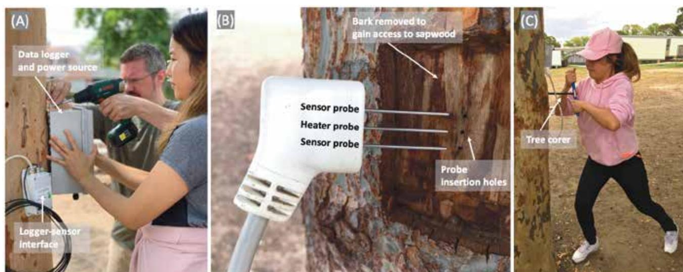
**FIGURE 12:** Tree water use work at the school. (A) Installation of data loggers and relevant auxiliary equipment. (B) Sensor head with probes before insertion into the stem; probe diameter is 1.25 mm. (C) Extraction of wood core to determine sapwood depth, moisture content and density. (A) Image© L. Vu; (B, C) Image © S. Pfautsch.
