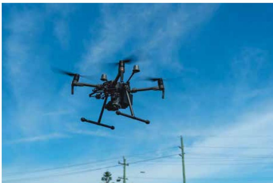
**FIGURE 11:** Matrice 210 RTK drone with FLIR XT2 camera for aerial assessment of surface temperatures. Image © D. Pataki.
