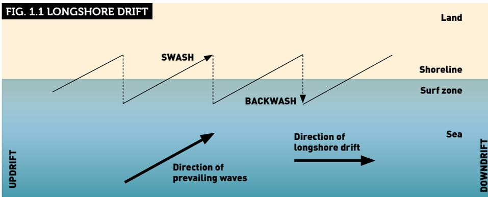
Waves approaching the beach at an angle cause a longshore current to form parallel to the shoreline. This longshore current can transport sand along the beach, from the updrift to downdrift direction. Figure adapted from the website page [bit.ly/2r00Qnd](http://bit.ly/2r00Qnd)
